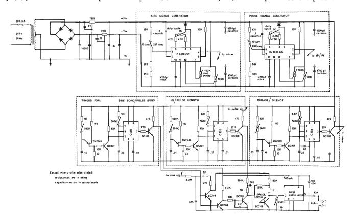
length and periods of silence between phrases (interphrase interval). The output of timer (iii) is to an 8", 8 ohm loudspeaker with frequency range 30 Hz - 4 K Hz, and power handling capacity 25W r.m.s., which resonates in free air at 30 Hz. The amplitudes of the sine and pulse song are regulated by a volume control.
